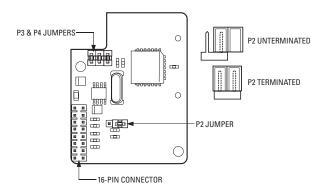
Figure 6. TXB-V Termination and Baud Rate (Bottom View)
